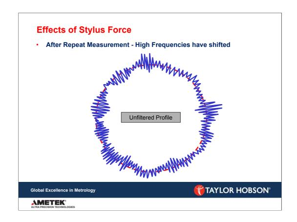
Here is the same component measured again this time the high frequency element has shifted.
