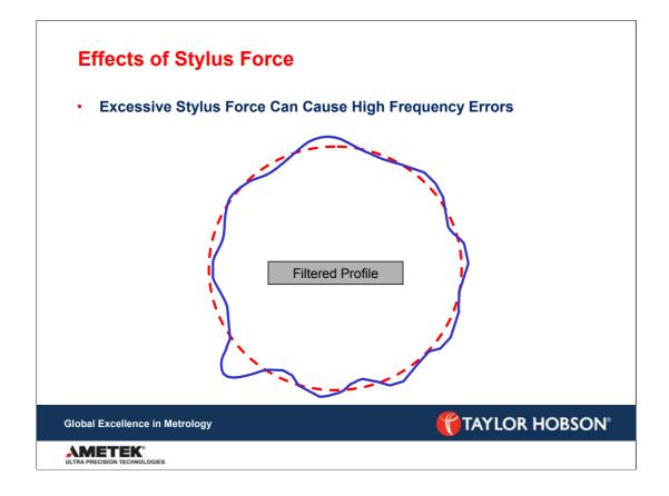
On measurements of fine surfaces or high precision surfaces a strong stylus force can cause high frequency errors.
