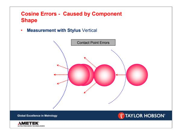
As can be seen above the arrows indicate the change in contact position of the stylus ball, in actual fact as the lobe passes through zero, contact will be made on the opposite side of the ball.
