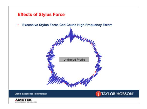
The errors shown here are due to the fact that both the stylus ball and the component are very smooth this causes a high frequency resonance.
