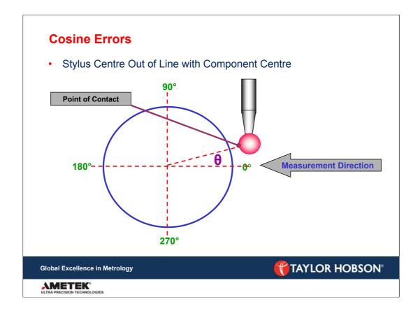
If we look at the situation here we can see that the stylus tip centre is not in line with the component centre along the measuring axis.
