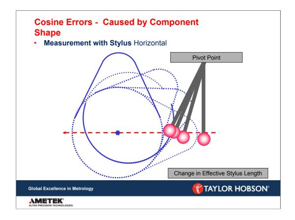
If the stylus is placed in a horizontal attitude we have a further error in that the effective stylus length is lengthening and shortening with respect to the component axis due to its pivotal movement.
