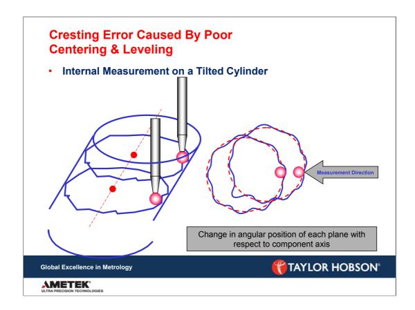
Other sources of error can be caused by bad centering and leveling of components.
