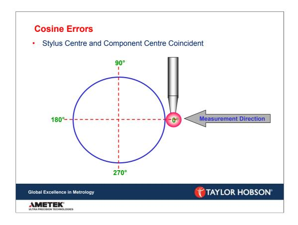
When measuring roundness the best possible means of measurement is when the stylus centre and the component centre coincide with the measuring direction.
