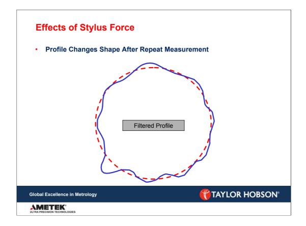
If the same component is measured again the shape will appear to change, this is because the effect is not repeatable and will appear at random on the surface.
