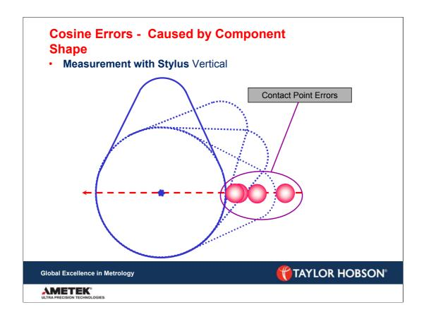
Sometimes the component shape can cause cresting or contact point errors.
