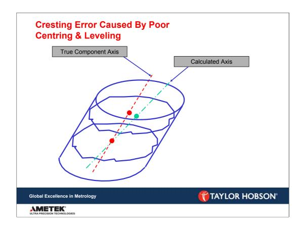
These incorrect centres will cause incorrect calculation of the position and tilt of the cylinder.
