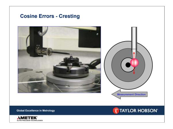
The standard is placed central on the table of the roundness measuring instrument and centered.
