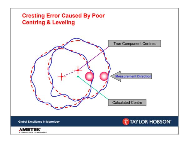
The above diagram shows the real centre of each component plane along with the assumed centre.
