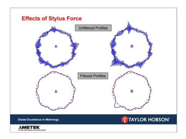
A good example of where this error may occur is on fuel injector bores where the surfaces are very fine, to remove this effect it is often best to reduce the stylus force to the minimum force possible.
