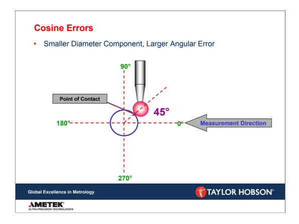
As can be seen above the smaller the component the larger the angular error in terms of cresting.
